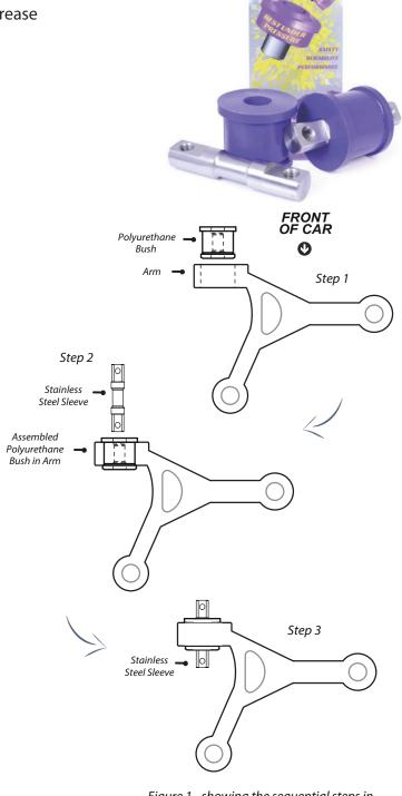
Figure 1 - showing the sequential steps in assembling this part in the arm
